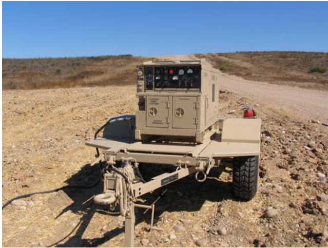
Figure 10: PU798 10KW generator trailer.
