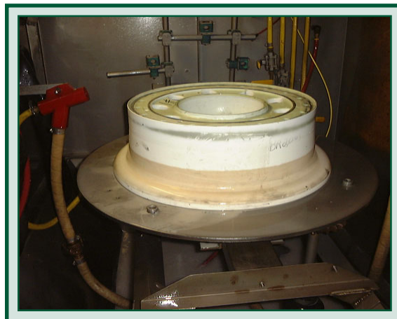
Aluminum oxide wet slurry blasting using 3/0 quartz
