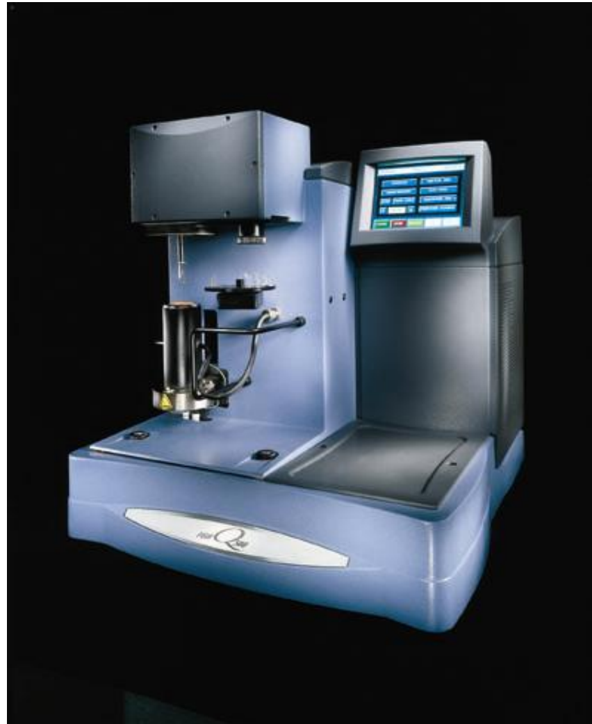
Figure 1. TA Vertical Microbalance with Evolved Gas Option Allowing Use as an Horizontal Wind Tunnel
