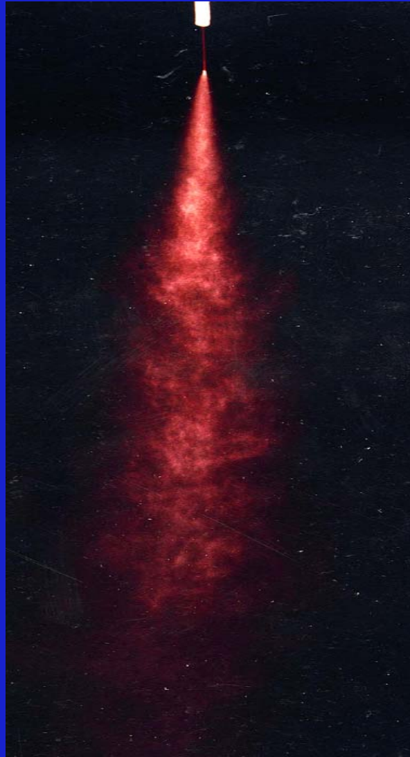
Aerosol spray of microbubbles and droplets generated by the CAN-BD process
