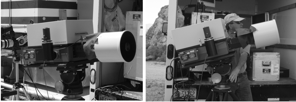
Figure 3.1: Two photos of the Bomem MR-254 Fourier Transform Spectrometer with the NFOV telescope at Edwards AFB, CA (see section 3.3). Also visible: the Canon XL-2 video camera used to document tests (left) and AFIT technician Greg Smith (right).
