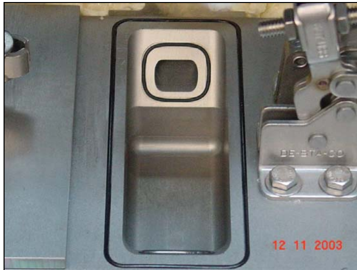
Figure 3. View from above the test cell showing the inlet port and sealing o-rings.
