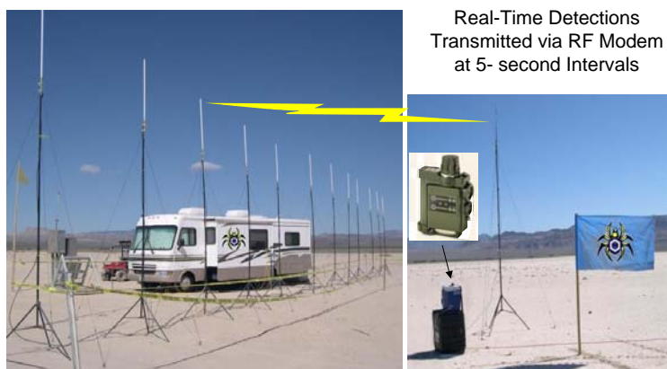
Figure 1: Typical test set-up of the data center and an element of the ground-based detection array.
