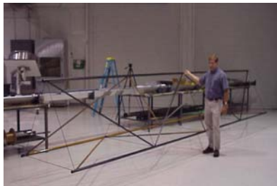
24-foot long truss, sub-Tg composite, weight: 9 lbs
