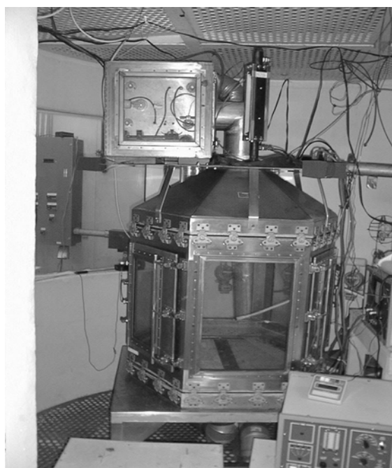
Figure 1. 750-liter experimental exposure chamber system.
