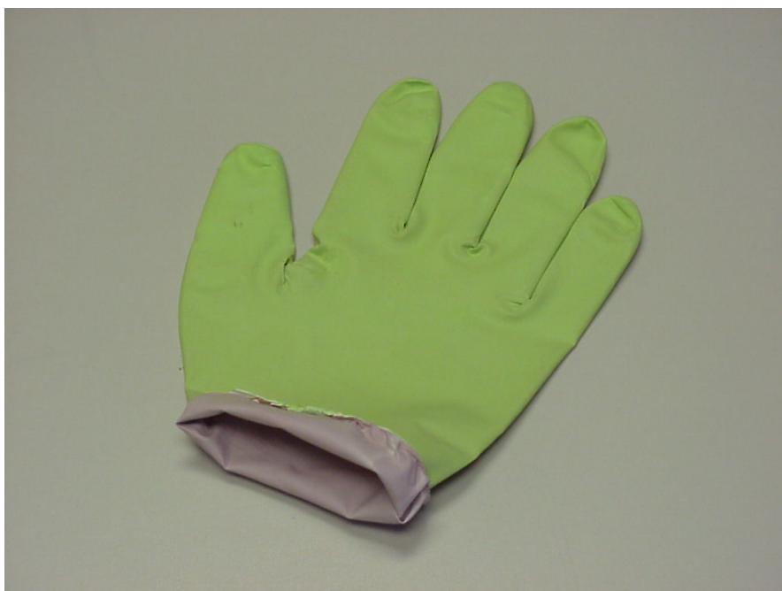
Figure 4. This glove, produced in Best Manufacturing’s research center, has a Neoprene outside layer, InMat’s Air D-Fense™ 2000R layer, and an inside layer of nitrile rubber. The pink color on the inside is due to the Air D-Fense™ 2000R, still visible through the nitrile rubber layer.
