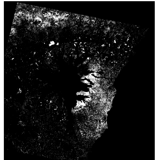
Figure 1: MYME2 step1: location of pixels presenting a decrease in vegetation cover from image N-1 (SPOT, 7 June 2001) to image N (L7 ETM+, 29 July 2001)
