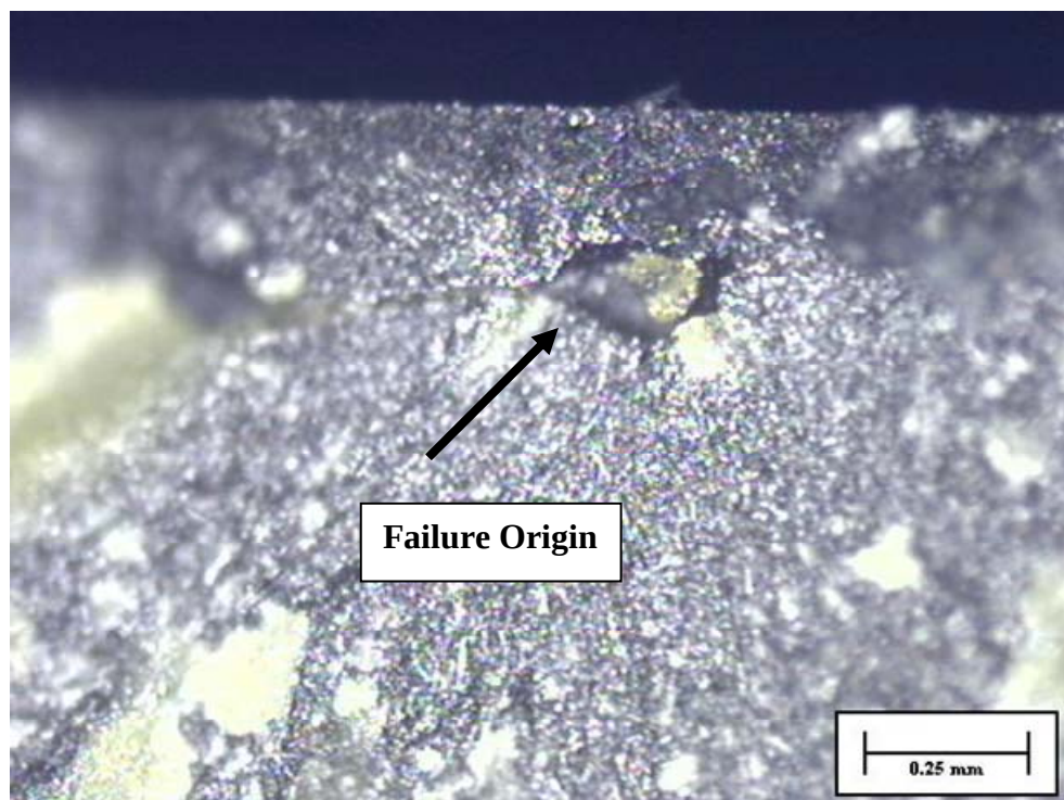
Figure 33. Fracture origin of specimen 5 from ITK4-4, side 2. Failure appears to have been caused by an agglomerate or inclusion of some sort.
