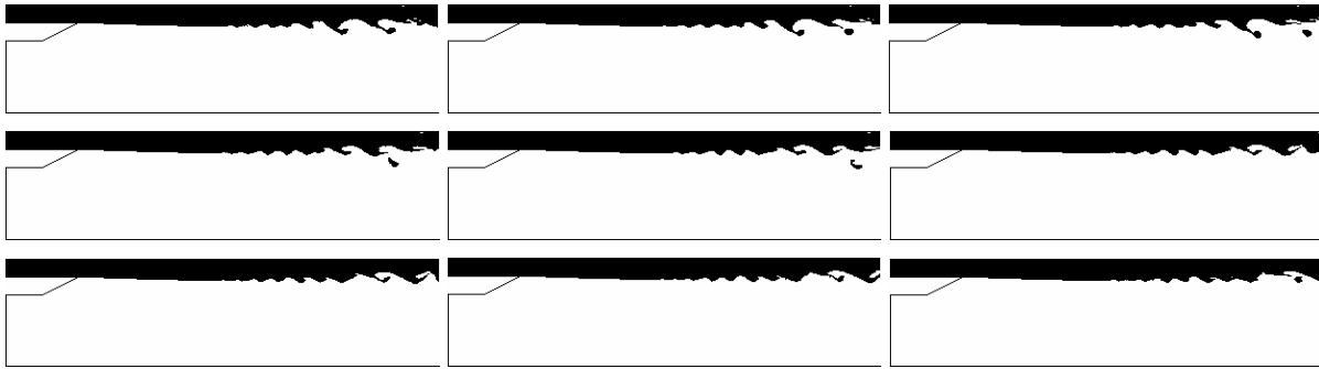
Figure 4. Axisymmetric simulation of the injector with a gas flow rate of 0.014 kg/s and an axial liquid velocity of 3.47 m/s. The black region represents the liquid. The flow is fully developed; images are given at 1.0 \times 10^{-4} s intervals from left to right and top to bottom. The simulation shown without artificial gravity is shown to better illustrate the stripping phenomenon.
