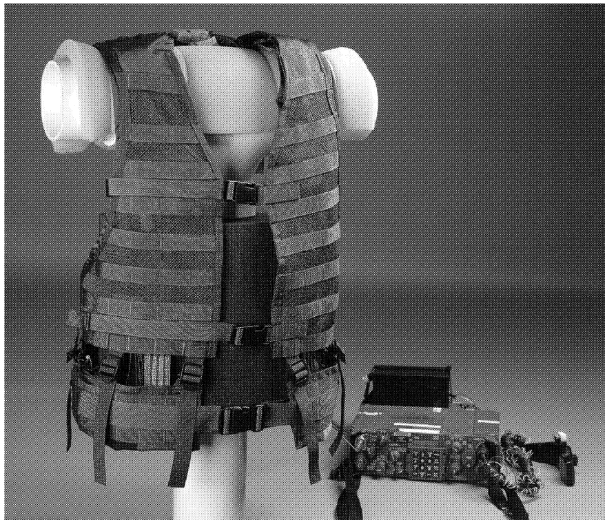
Figure 1. Prototype Wearable Body-Borne Antenna/Radio
