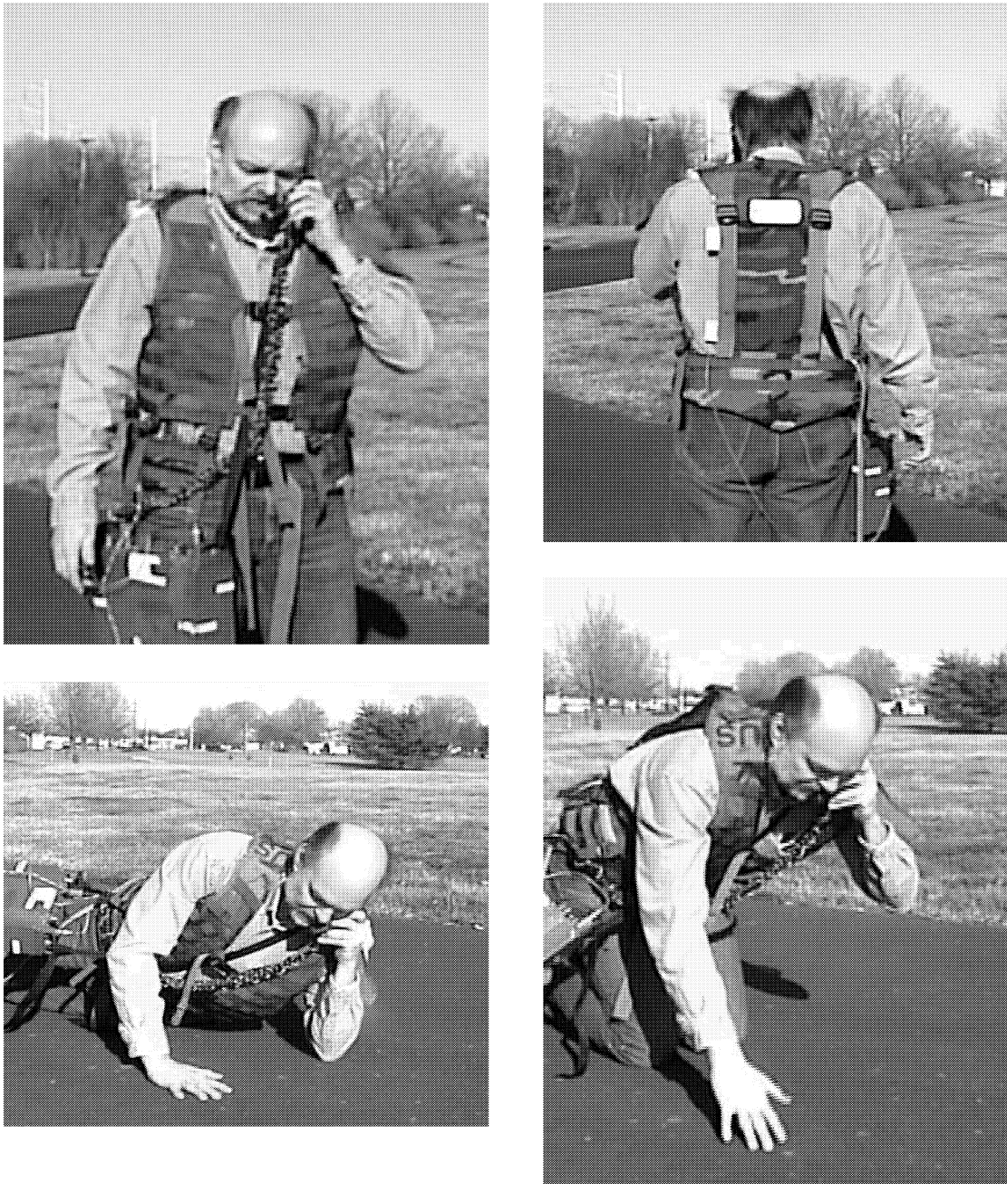
Figure 34. Wearable Antenna Tested in Various Positions
