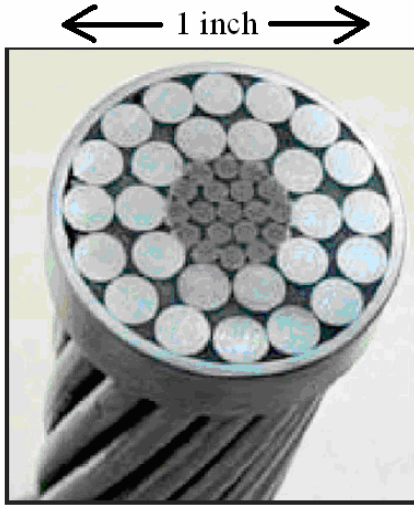
Figure 12. The cross-section of a power line; conducting aluminum members surround a supporting steel core (ORNL 2003).
