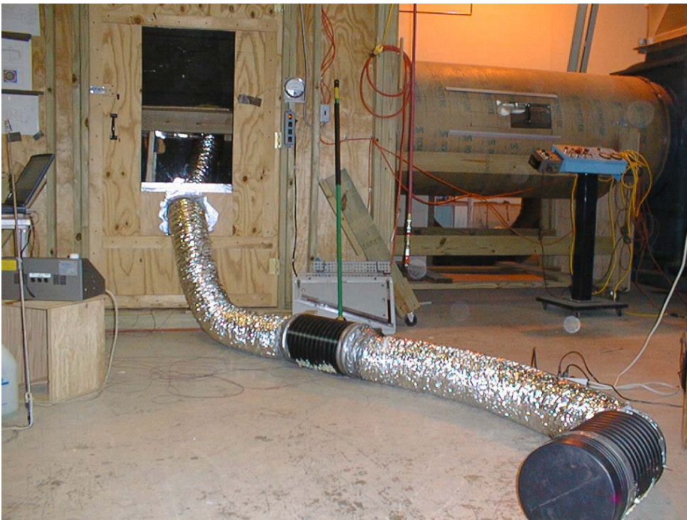
Figure 2. The model gopher tortoise burrow extended through door of the wind tunnel test section with entrance facing 90^\circ to wind direction. Each section of black corrugated pipe contains an aerosol sensor. Those at the 3-m and 5-m positions are visible here. The 1-m position is within the chamber.
