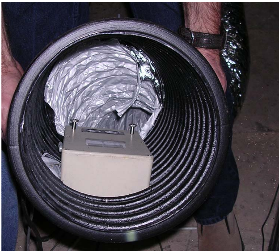
Figure 7. RAS mounted in plastic drain pipe mounted at end of model gopher tortoise burrow.
