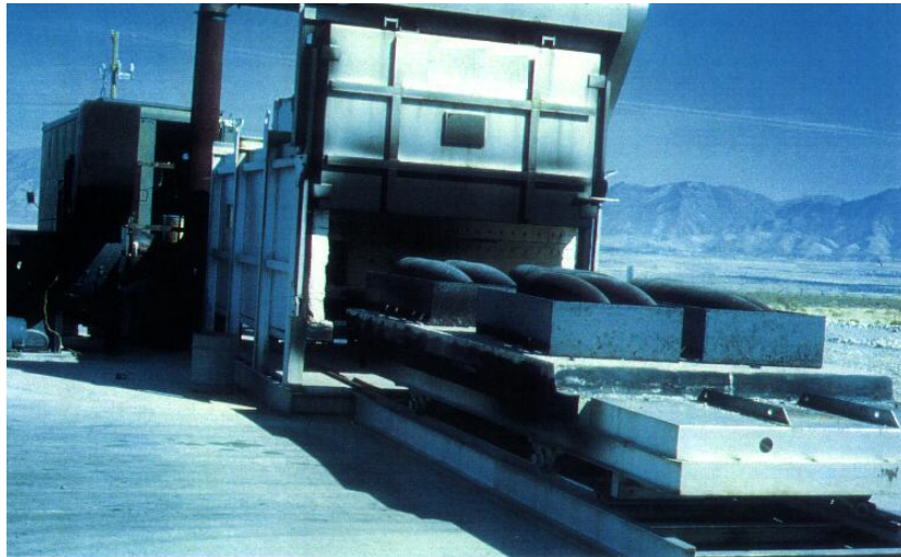
Figure 1. The U.S. Army Simple Flashing Furnace with a Rolling Hearth (shown here processing 750 lb bomb shells).
