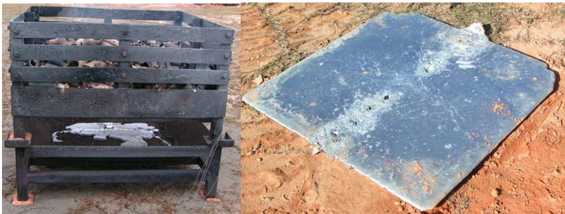
Figure 8. Basket CC1 Immediately Following a Test. (Note the molten material that has collected in the catch basin. An aluminum ingot from a subsequent test is off to the right.)
