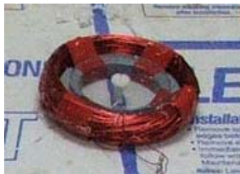
Figure 6. Photograph of a receive loop antenna.
