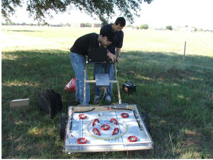
Figure 26. Complete one-man-portable EMI system prototype.
