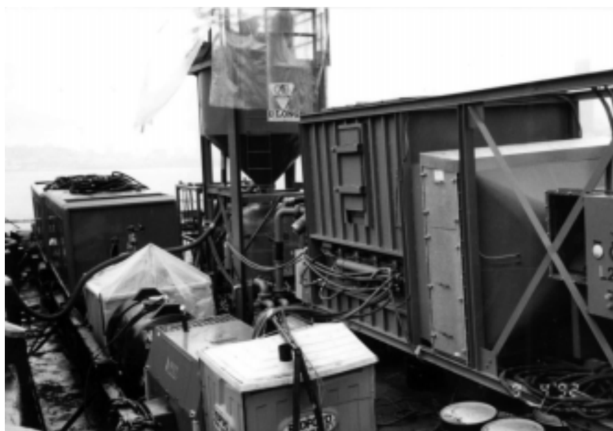
Figure 3-7: Set-up for Steel Grit Recycling (Courtesy of Long Painting Company)
