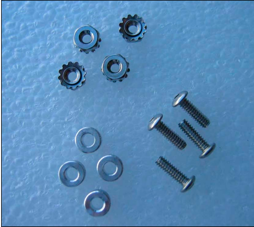
Figure IV-5. Screws, spacers, and lock nuts used to assemble FO module onto PCB card.
