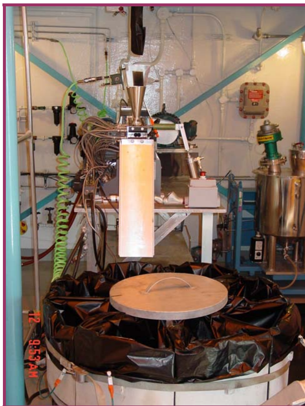
Figure 35. Photo of 19-mm TSE Setup for MTTP Extrusion, Including Collection Turntable.
