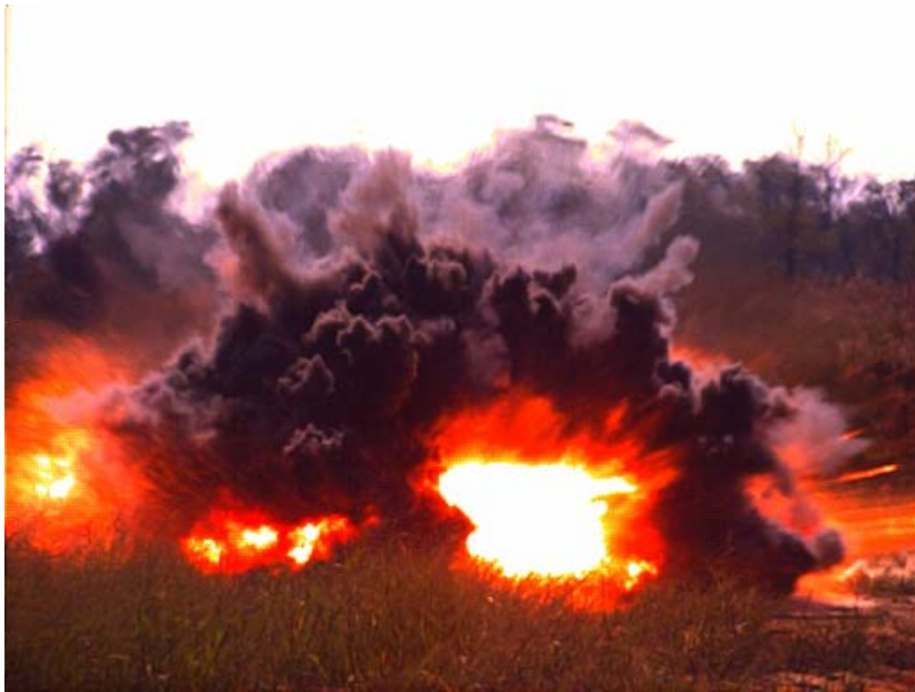
Figure 4.7. Close-Up View of Fireball Formed During Test of High Explosive 4.2 in. Mortar Round (Over Hard Surface)
