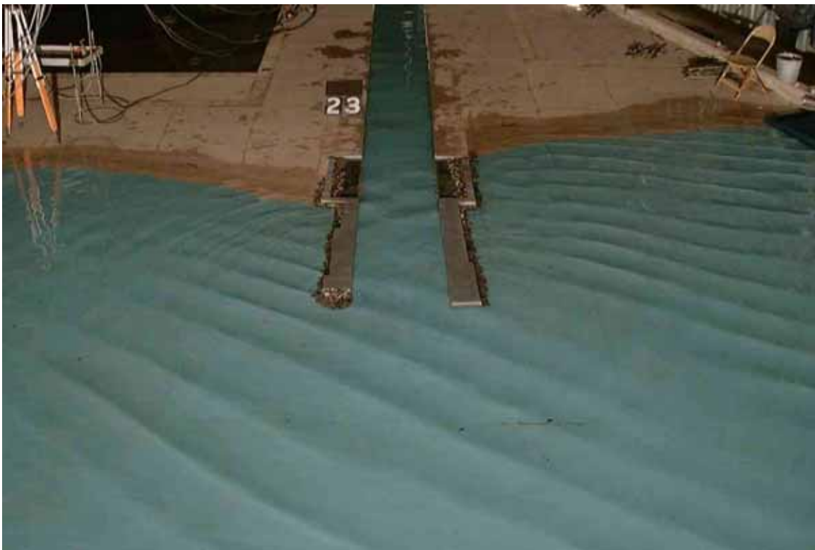
Photograph 5b. Typical wave patterns for existing conditions; 5-sec, 1-m waves from 45 deg North; swl = +0.9m LWD.
