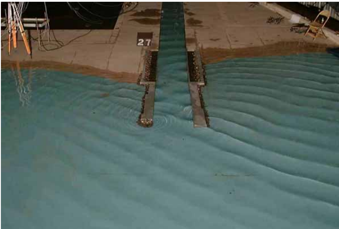
Photograph 35b. Typical wave patterns for Plan 5; 5-sec, 1-m waves from 45 deg North; swl = +0.9m LWD.
