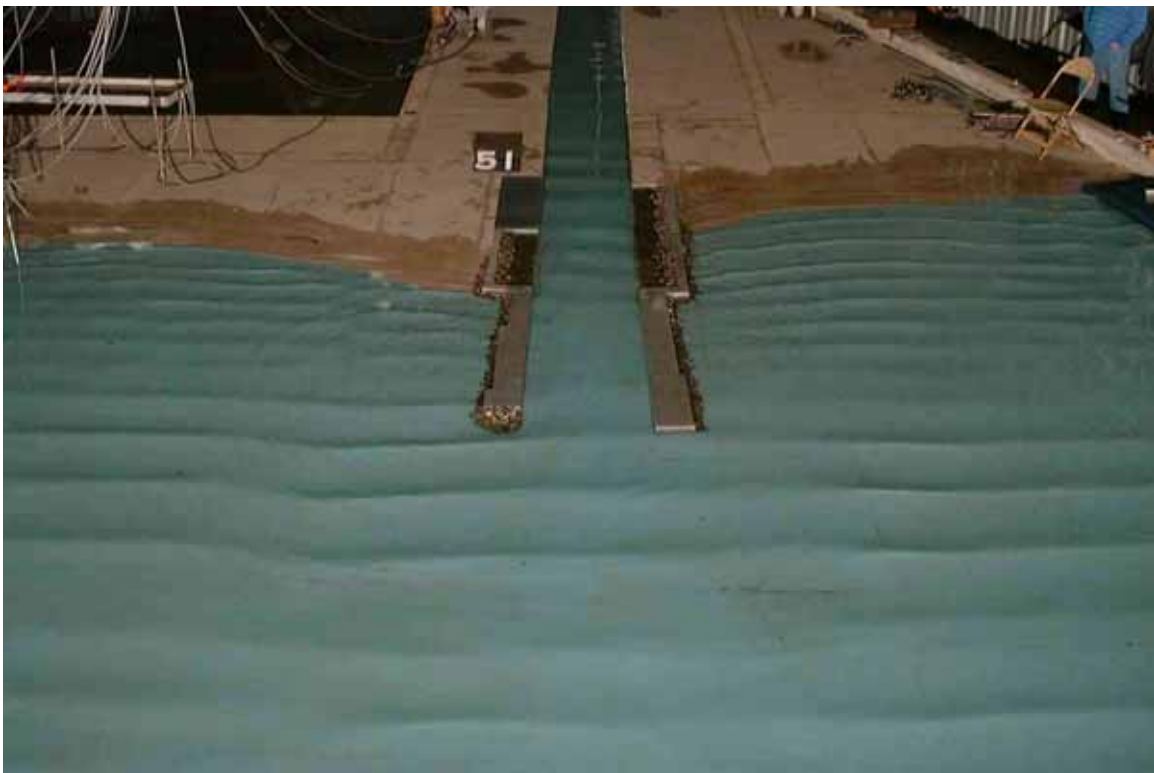
Photograph 45b. Typical wave patterns for Plan 7; 5-sec, 1-m waves from 0 deg; swl = +0.9m LWD.
