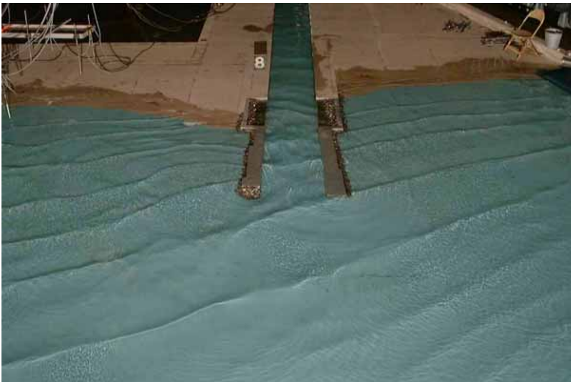
Photograph 2b. Typical wave patterns for existing conditions; 8-sec, 2-m waves from 45 deg South; swl = +0.9m LWD.
