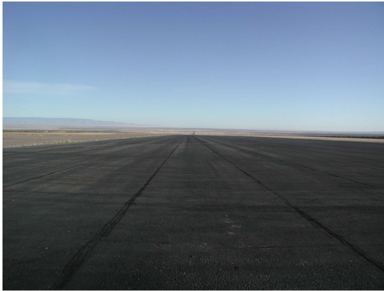
Figure 3.15: This photo is taken looking downrange at NRTF, and gives a good perspective of the rise in elevation which contributes to the clutter problem.
