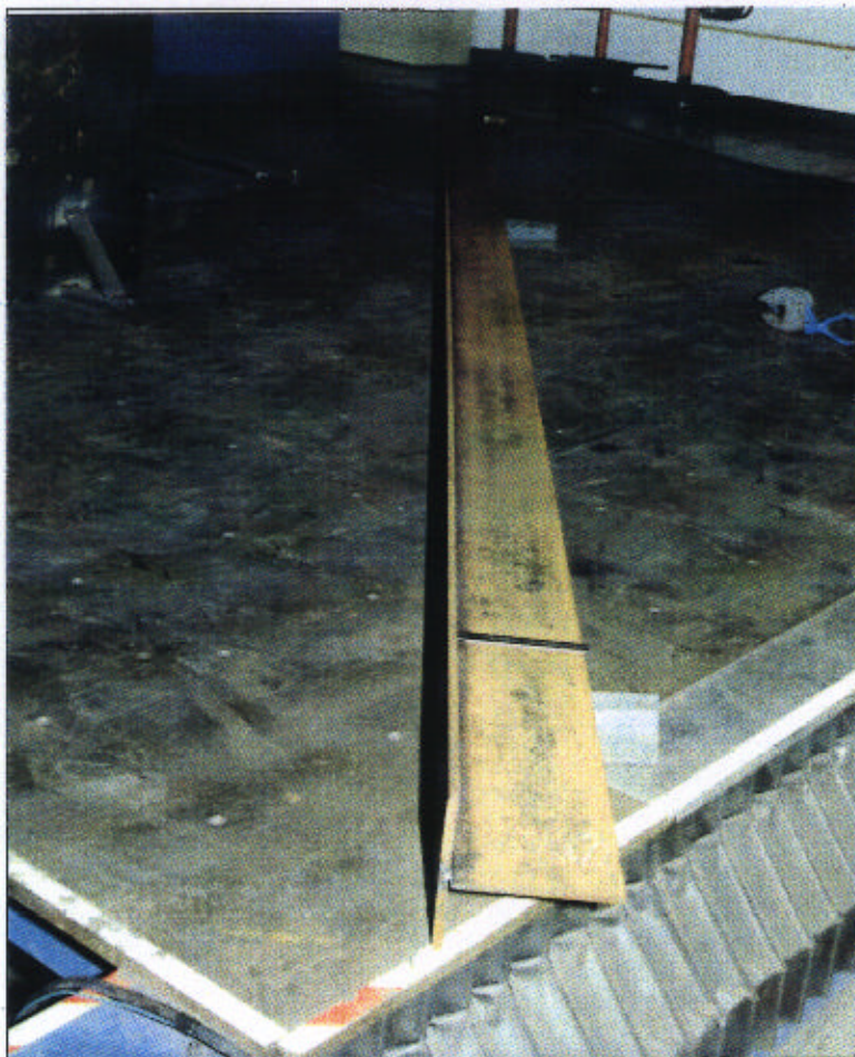
24. Tee section made of 3/8x6 inch flat bars, autogenous weld
