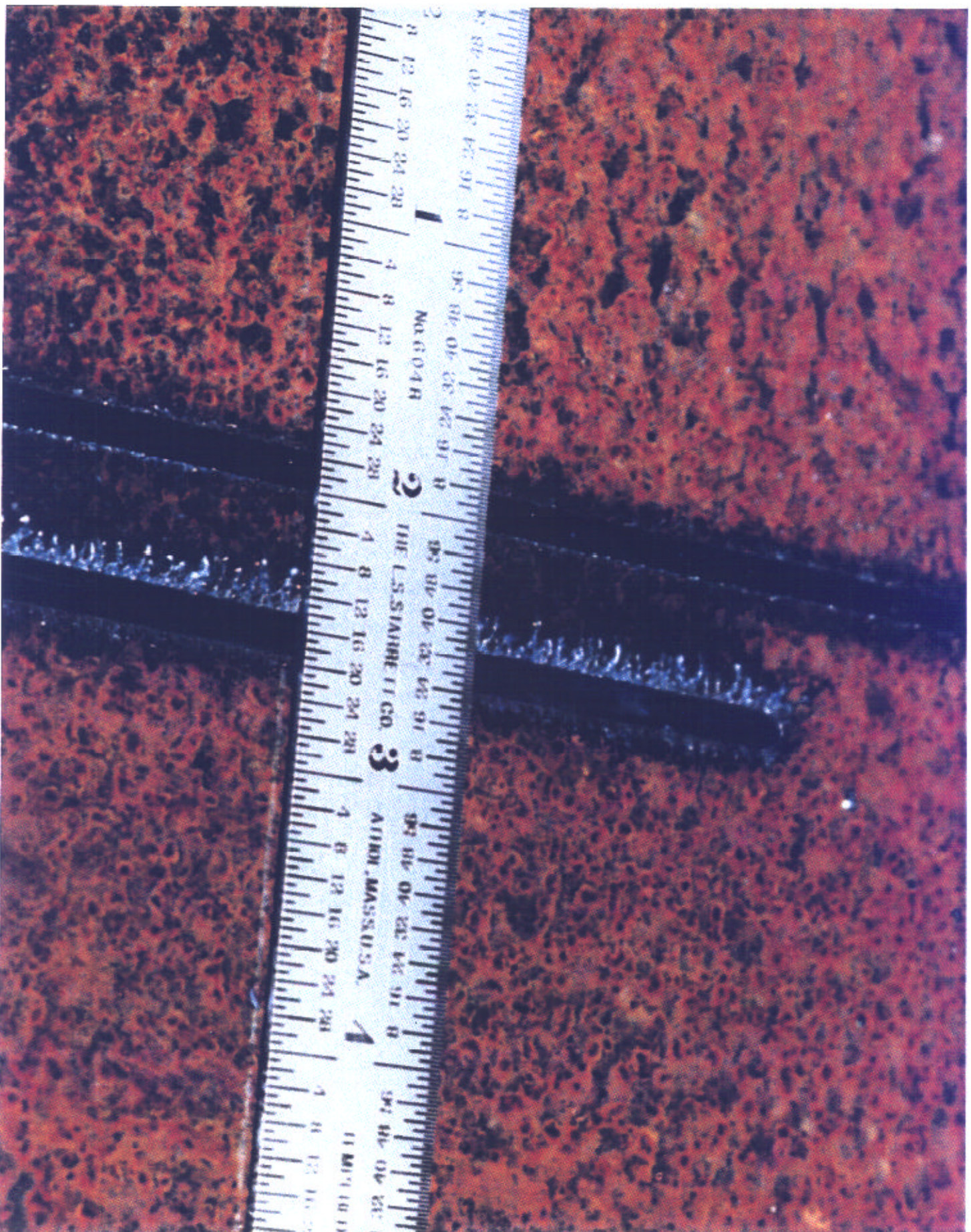
19. Kerf width of simultaneous plasma test cuts on W6x20 beam
