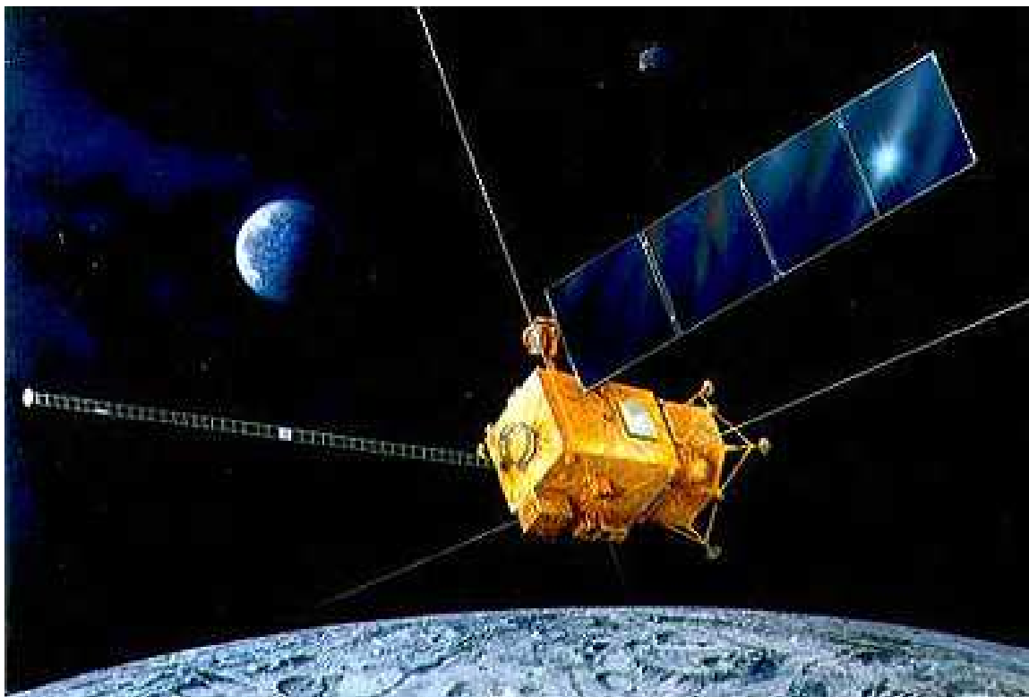
Figure 2.1: SELENE Orbiter. The spacecraft has three components: the main orbiter, a small relay satellite, and a small Very Long Baseline Interferometry (VLBI) satellite. The main orbiter, which has a rectangular box shape, carries the scientific instrumentation. The relay satellite is an octagonal shape and will be used to communicate between the orbiter and Earth. The VLBI satellite is the same shape as the relay satellite; its purpose is to conduct investigations on the position and precession of Earth's moon [24].
