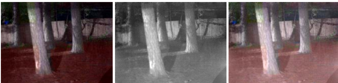
Figure 44: Results from chrominance transfer. Left: UV chrominance transfer from the RGB to the SWIR image. Center: SWIR image interpolated with the RGB boundary conditions. Right: Chrominance transfer from the RGB image to the interpolated image.
