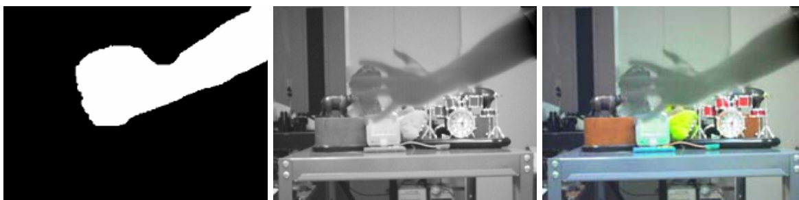
Figure 38: Improved chrominance transfer using non-rectangular interpolation boundary conditions. Left: The mask defining the boundary condition. Center: The interpolated SWIR image. Right: Chrominance transfer from the RGB image to the interpolated image.
