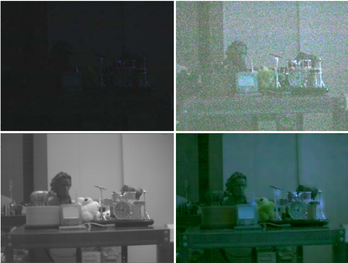
Figure 56: Inputs and output of our multi-spectral bilateral fusion technique on a video frame. Upper Left: Original RGB frame; Upper Right: Histogram stretched original RGB frame; Lower Left: Corresponding SWIR frame; Lower Right: Multi-spectral bilateral fusion result.
