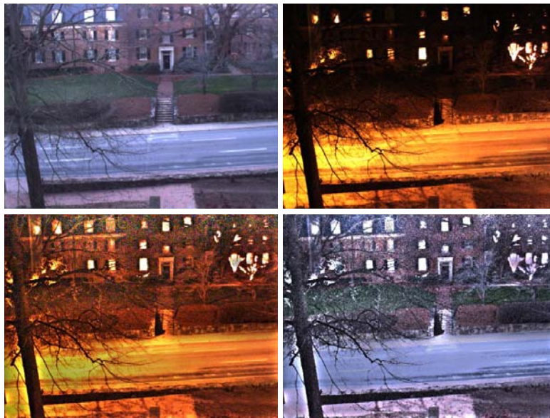
Figure 15: Poisson interpolation with boundary conditions from a daytime image taken with the same camera. Upper Left: daytime RGB image, Upper Right: long exposure nighttime RGB image, Bottom Left: long exposure gradient field interpolated with daytime boundary conditions with nighttime chrominance, Bottom Right: same as Bottom left with daytime chrominance
