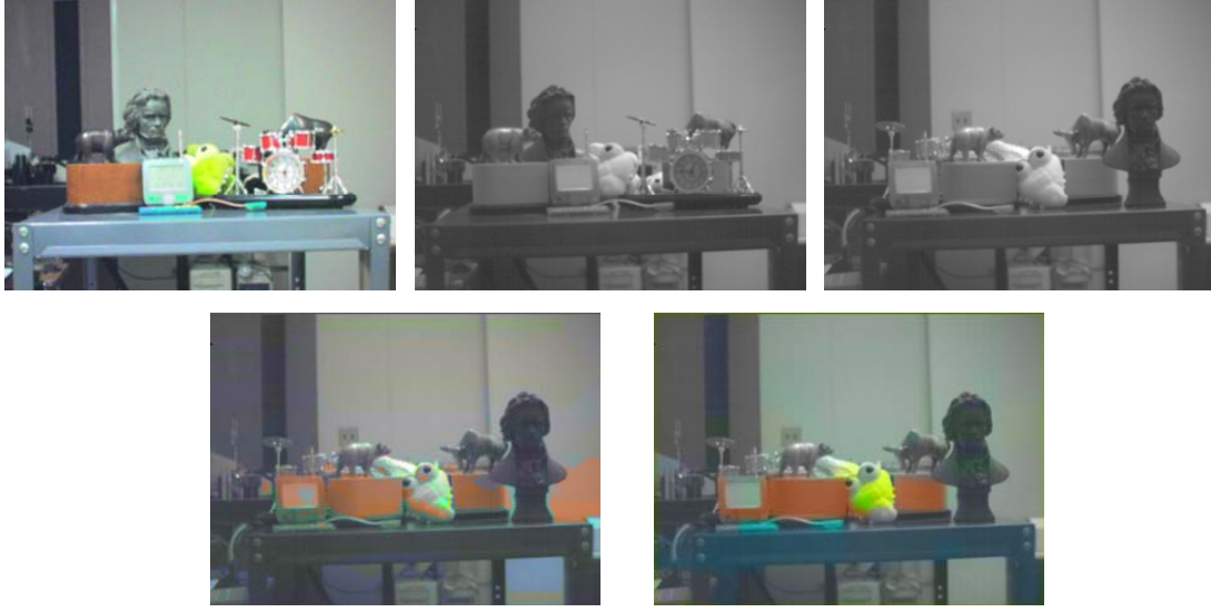
Figure 49: Colorized SWIR image based on a pair of examples. The top left and top middle are the source image pair of a registered RGB image and a grayscale SWIR image. The top right is the target SWIR image. The bottom left is the colorized result based on mean and variance. The bottom right is the colorized result using our belief propagation-based technique.
