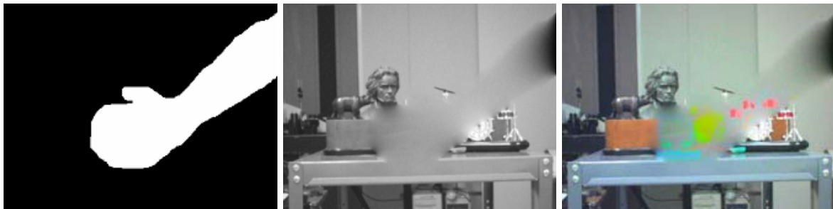
Figure 41: Chrominance transfer using non-rectangular interpolation boundary conditions. Left: The mask defining the boundary condition. Center: The interpolated SWIR image. Right: Chrominance transfer from the RGB image to the interpolated image.
