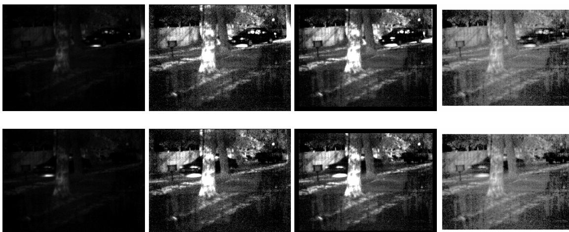
Figure 29: Two frames of SWIR video depicting a car with no headlights. From left to right: the original frame, a histogram stretched version of that frame, the frame histogram stretched and processed with ASTA, and the frame processed using our full ASTA and tone mapping pipeline
