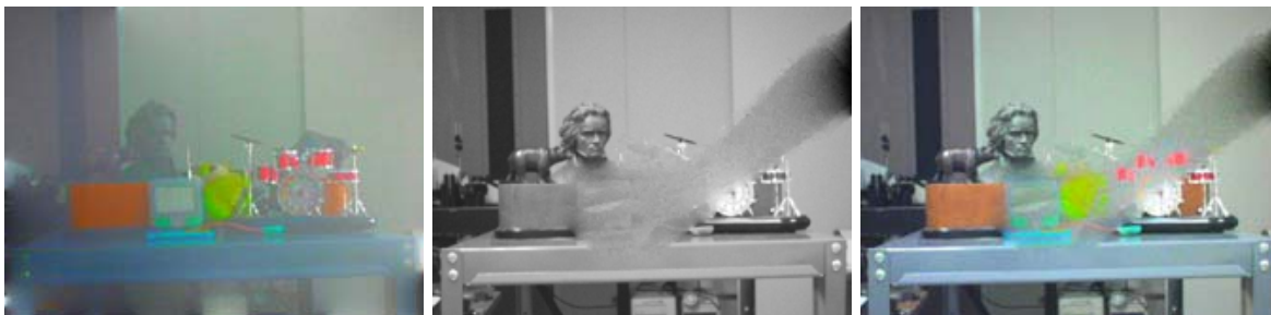
Figure 42: Results from a somewhat brighter “dark” image. Left: UV transfer to an interpolated image using rectangular boundary conditions. Center: Interpolation of an arm from the dark scene into the bright image. Right: UV transfer from the RGB image to the interpolated image.
