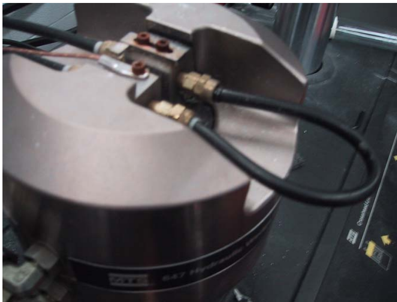
Figure 14. Tubes for Cooling Water Connected to Hydraulic Wedge Grips
