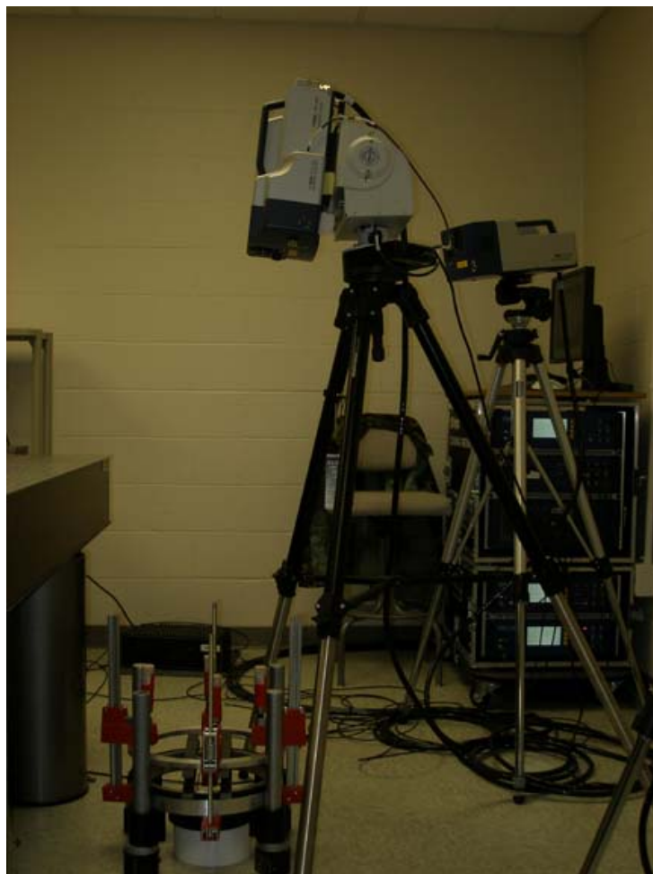
Figure 44: Laser Vibrometer Test Setup
