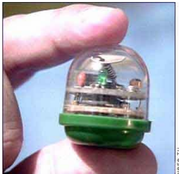
Figure 18. Gumball Size Wireless Sensor Pod
