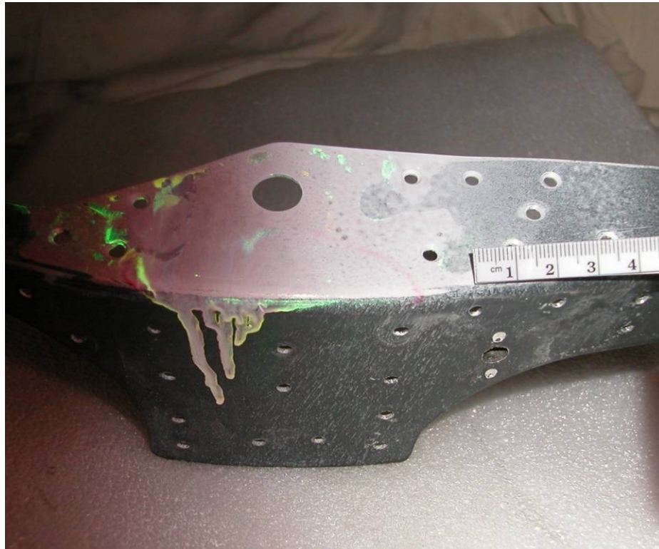
Figure 3. Fluorescent indication of the crack on side B.
