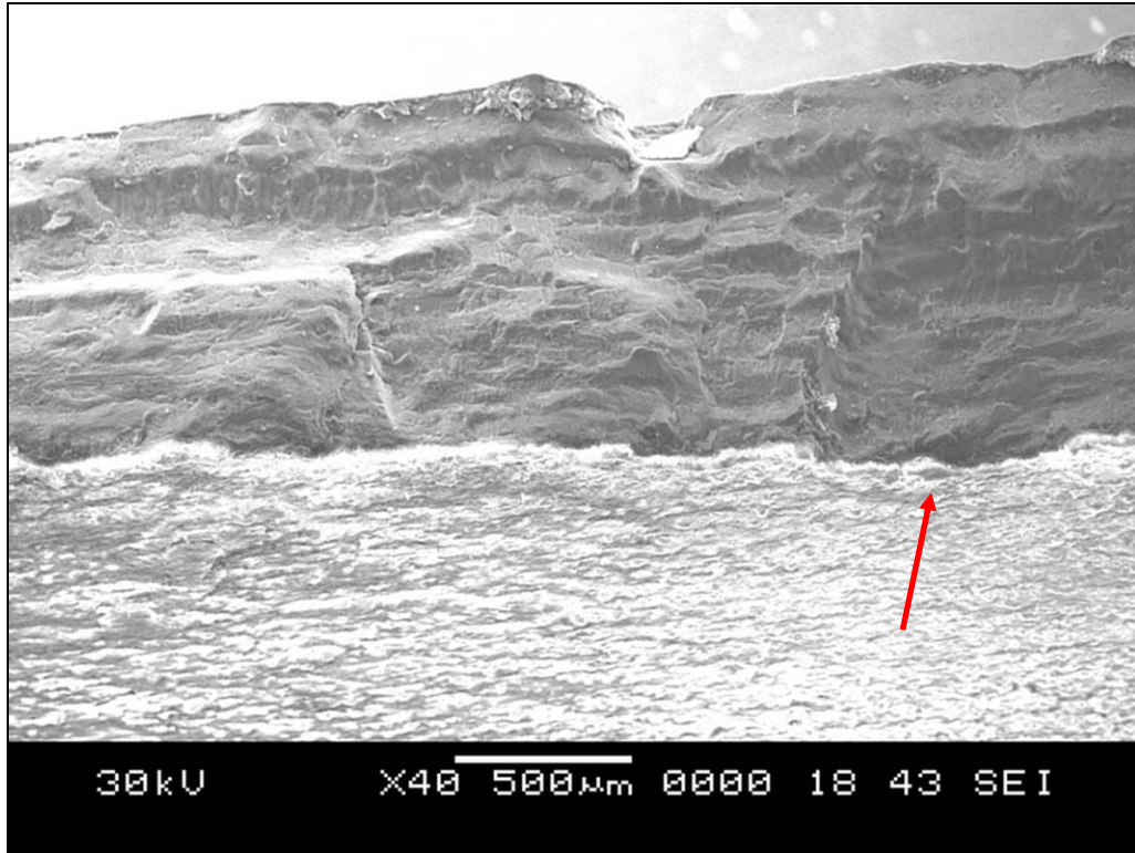
Figure 19. SEM micrograph of the center fatigue initiation site at 45°.
