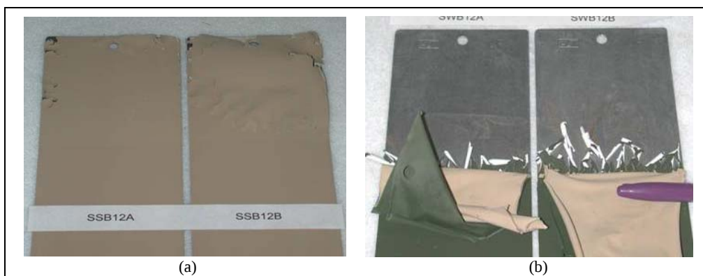
Figure 10. MIL-C-53039 CARC (a), MIL-DTL-64159 Type II CARC (b), both shown after 30-min immersion in Gardostrip Q7900.
