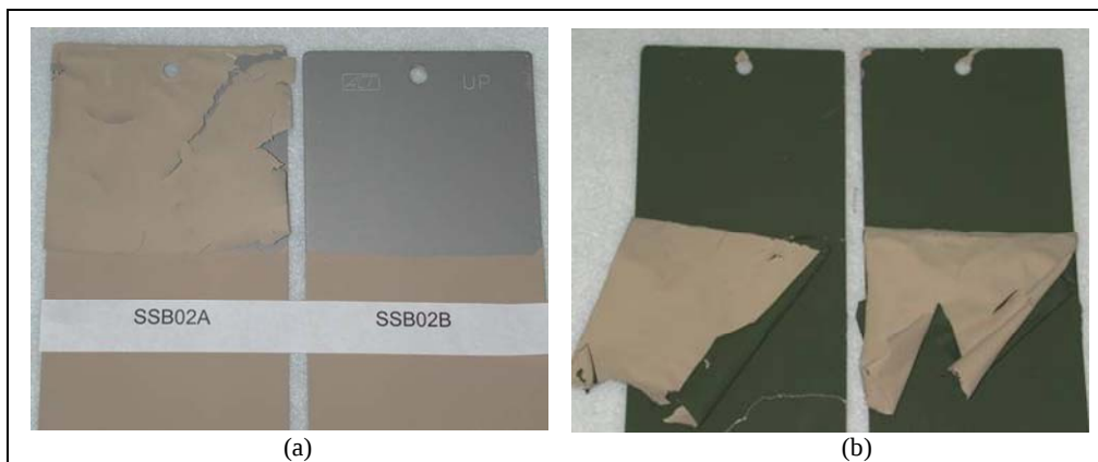
Figure 11. MIL-C-53039 CARC (a), MIL-DTL-64159 Type II CARC (b), both shown after 30-min immersion in straight methylene chloride.
