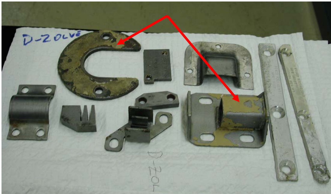
Figure 31. Stripping of miscellaneous parts after 30-min immersion in D-Zolve 298. With the exception of the two parts shown (see arrows), all of the paint was removed, and parts were free of corrosion. Paint was left on only one side of the C-flange (shown).
