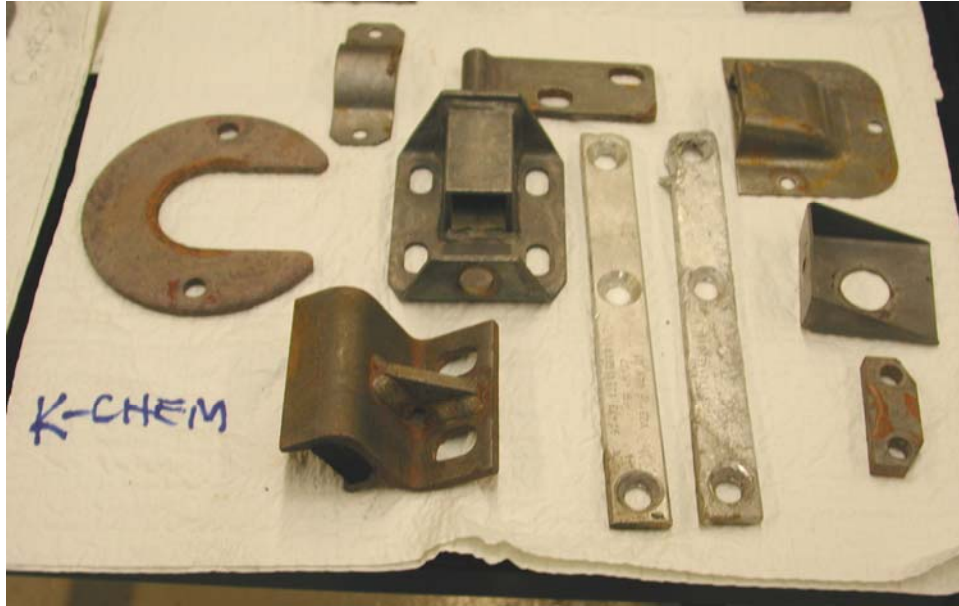
Figure 30. Stripping of miscellaneous parts after 30-min immersion in K-Chem CARC Stripper III. One hundred percent of the paint was removed; however, some light corrosion on the steel parts was generated.
