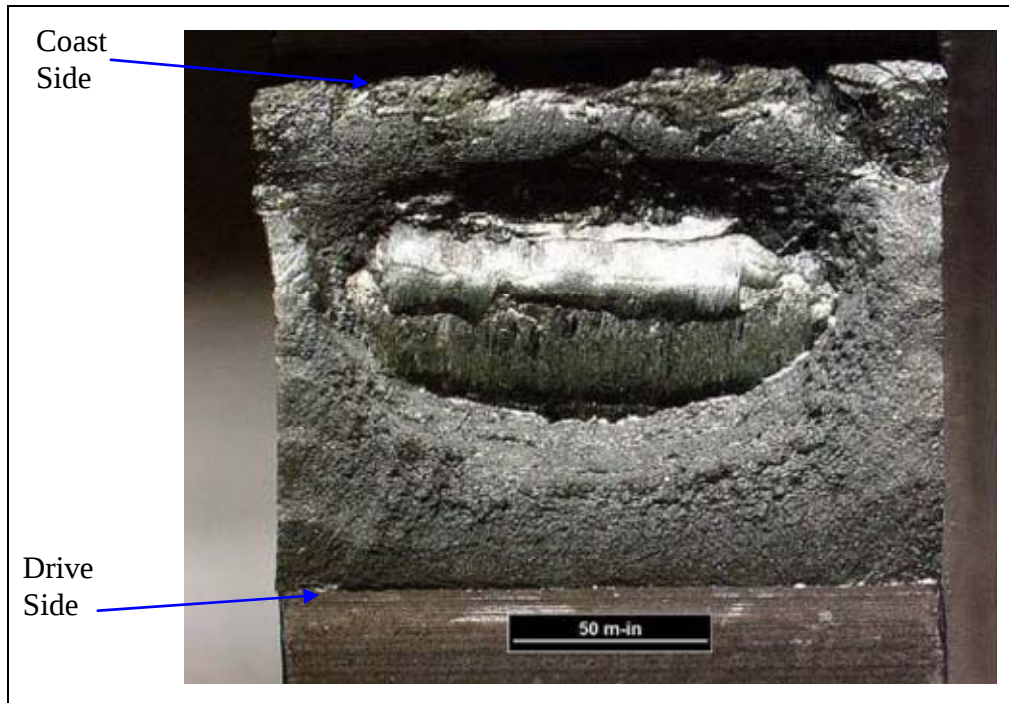
Figure 19. Tooth 31, gear fracture half.
