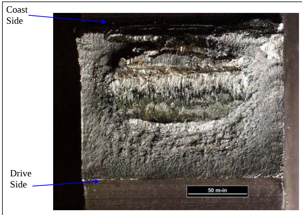
Figure 17. Tooth 30, gear fracture half.
