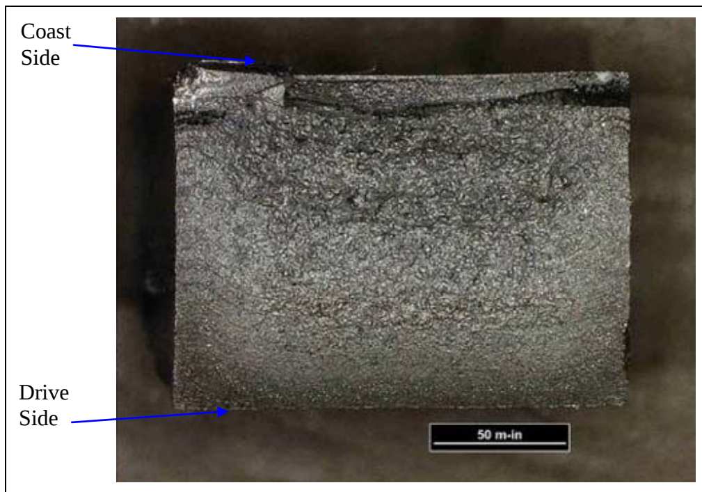
Figure 14. Tooth 29, tooth fracture half.
