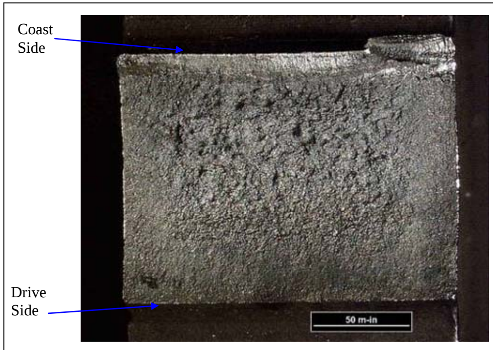
Figure 15. Tooth 29, gear fracture half.
