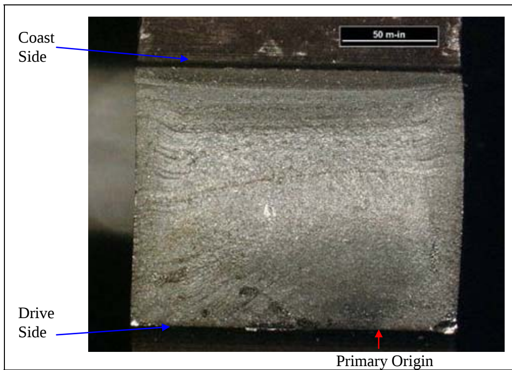
Figure 3. Tooth 1, gear fracture half.
