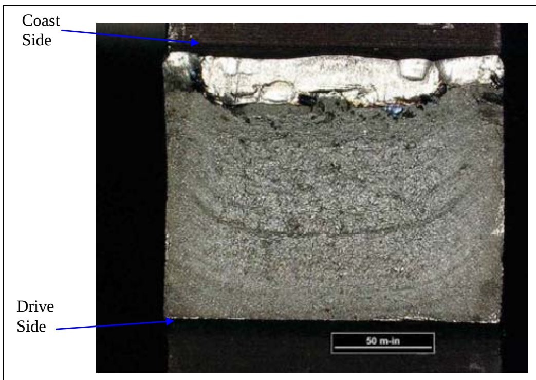
Figure 9. Tooth 3, gear fracture half.
