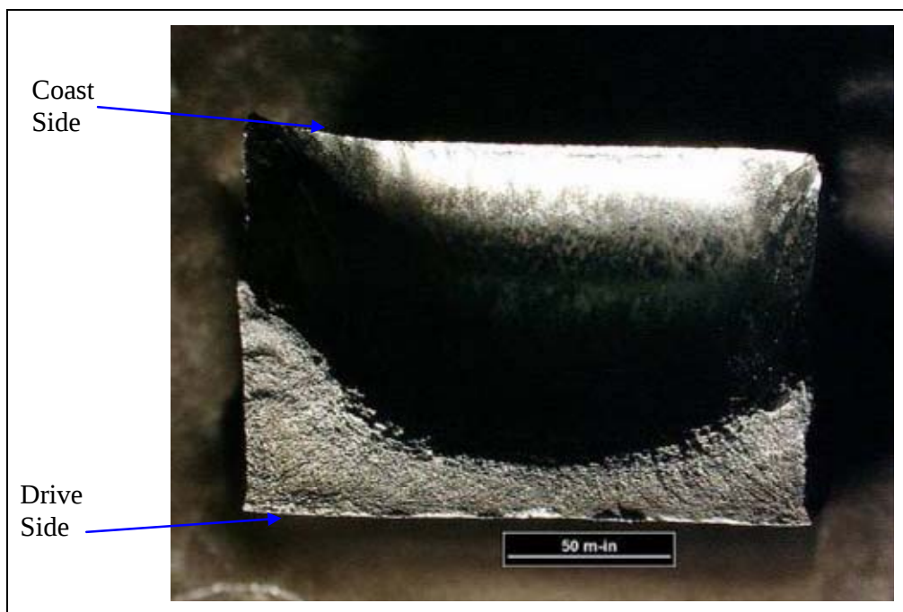
Figure 18. Tooth 31, tooth fracture half.
