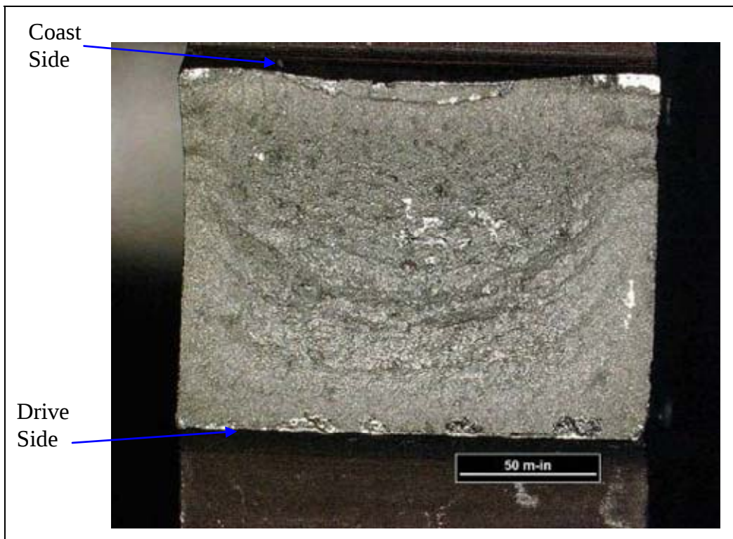
Figure 11. Tooth 4, gear fracture half.
