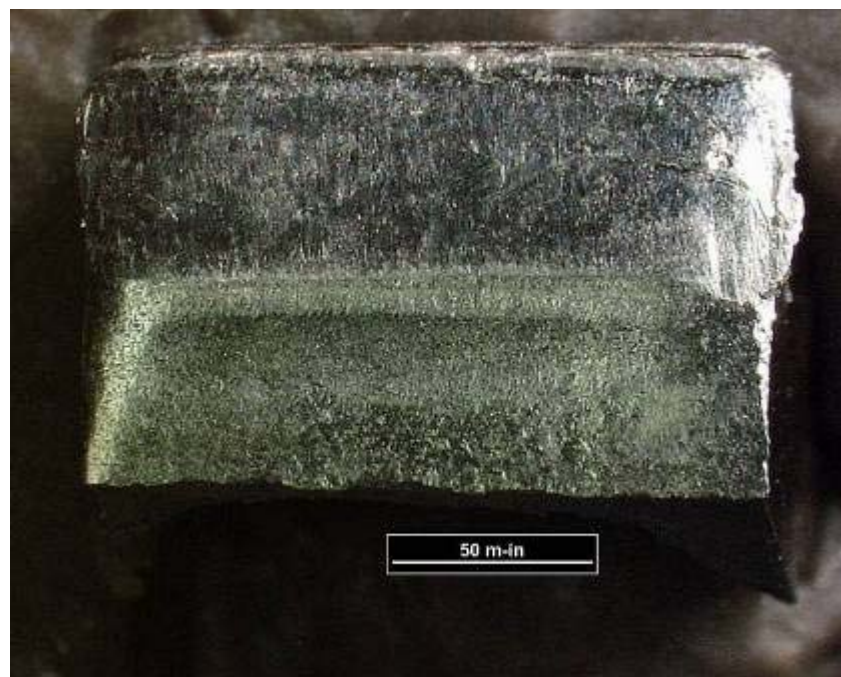
Figure 26. Drive side, tooth 31. (Note: worn adjacent to fracture surface.)
