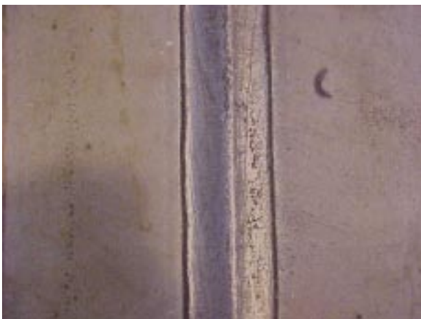
Face Reinforcement -- Blocks 314 / 400 FIGURE 6-15
