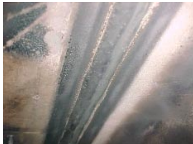
Root Reinforcement -- Blocks 314 / 400 FIGURE 6-16
