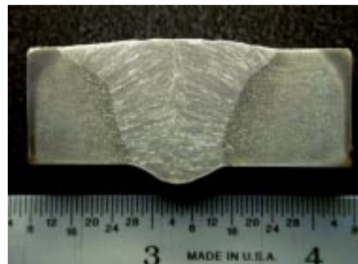
3/16" ROOT GAP / 45° INCLUDED V-GROOVE FIGURE 6-2 TEST NO. 397 (WPS) NP-7A2.6C
