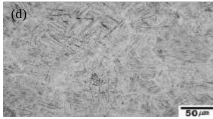
Fig. 10 Optical micrographs of (a) As-received, (b) FC, (c) AC and (d) WC specimens.
