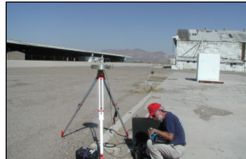
c. Established differential GPS base station used for precise trajectory information during LiDAR surveys.
