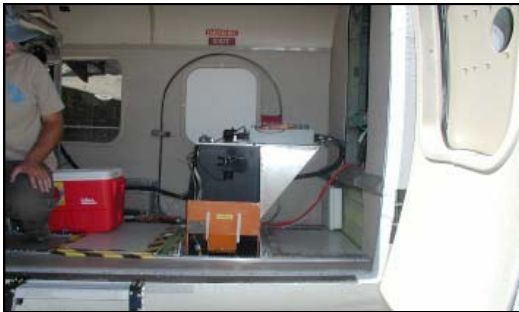
b. ATM-IV instrument mounted within the Twin Otter aircraft.
