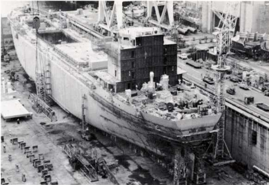
FIGURE 3-53: Erection Level. Finish paint was applied to the undersides of hatch-covers before the hatch cover/coaming assembly was fitted on-board. Keel plus 28 workdays.
