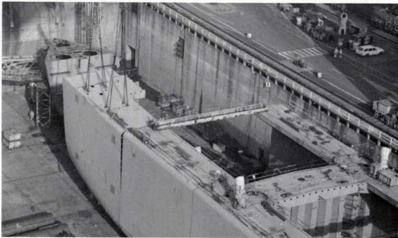
FIGURE 3-49: Erection Level. Landing the grand block shown in Figures 3-33 and 3-34. Keel laying plus 22 workdays.
