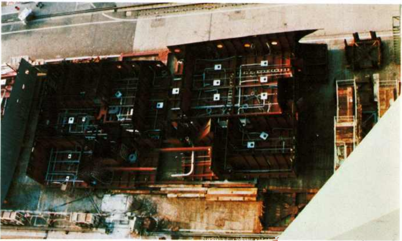
FIGURE 3-42: On-block Outfitting Level. Zone, area and stage are the same as in Figure 3-41. The blocks are different.
