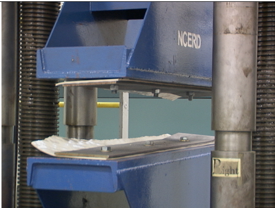
Figure 4.6 – Failure of Polymer Sample
