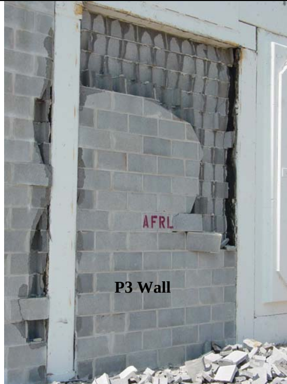
Figure 5.27 – CMU Wall Retrofitted with P3 Polymer after Explosion
