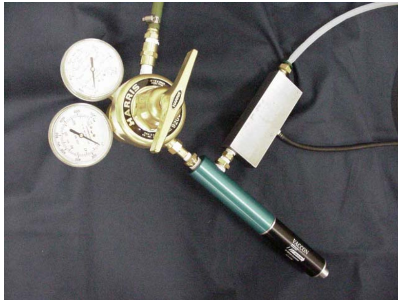
FIGURE 17. VENTURI PUMP, INLET PRESSURE REGULATOR, STATIC PRESSURE TAPPINGS, SMALL BORE TUBE, AND DIGITAL MANOMETER
