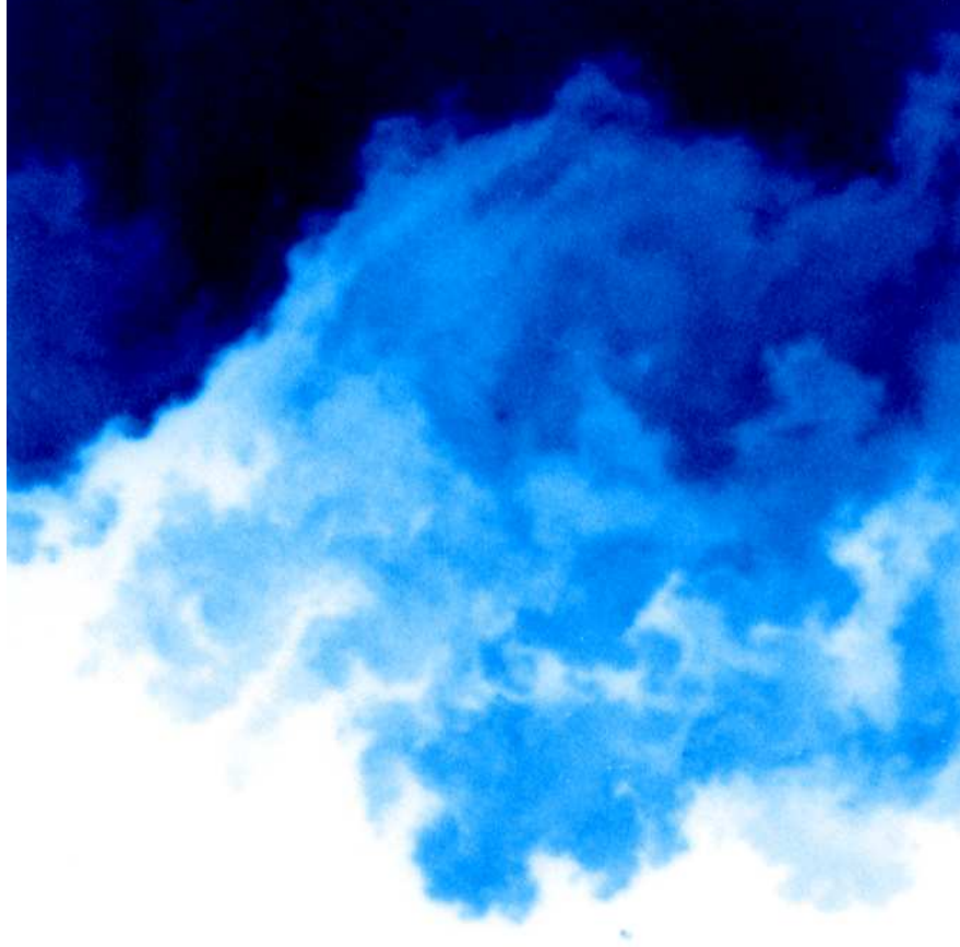
Figure 9: Results of the evolution (top) of the optical path difference (OPD) for wavefronts propagating through the refractive field (bottom) of the high Reynolds number compressible separated shear layer, using the image data in figure 6 reproduced here for comparison. Successive OPD profiles are shown at several transverse distances through the flow, with the wavefronts propagating vertically from bottom to top.
