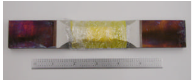
Figure 1e: A thick section specimen with salt solution soaked tissue wrapped around the gage section.
