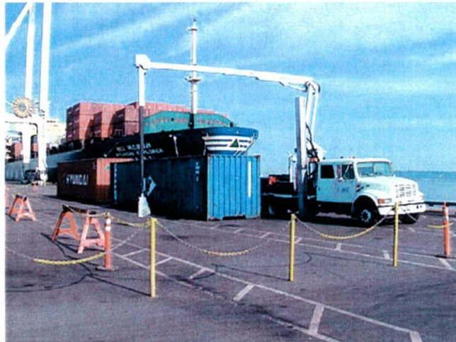
Figure 1-4. Mobile VACIS in use, inspecting containers at a port (Americana Impex Consulting Co, 2003).
