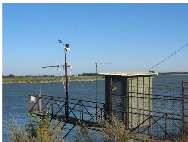
Fig. 1. RiverSonde installation at Threemile Slough. The RiverSonde antenna is mounted on the left side of the walkway and is over the water about 4 m from the bank. The weather station sensors are above the antenna. The smaller antenna is for USGS data telemetry. The USGS and RiverSonde equipment are inside the shelter.
