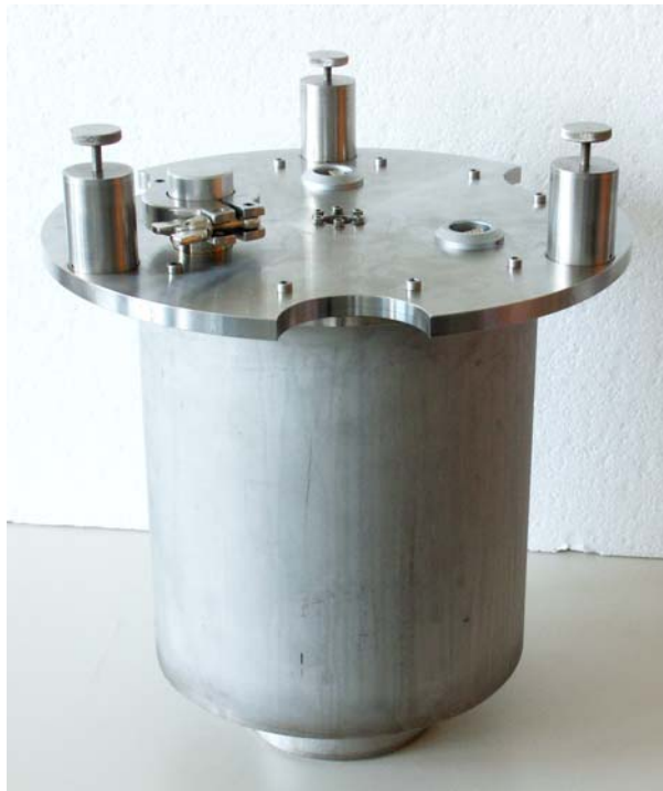
Figure 2.2-3 Completely Assembled Vacuum Chamber
