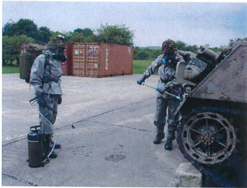
Figure 6 Decontamination in impermeable suits. First the tank was sprayed using the can on the left below, then the tank was scrubbed.
