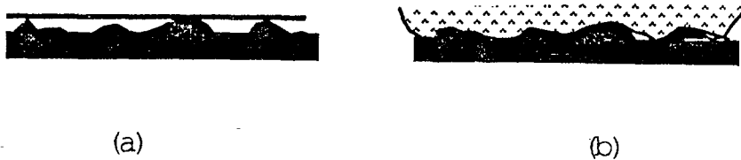
Figure 2.2: (a) Rigid contact with an irregular surface results in contact at a number of discrete points only. (b) Compliant contact with an irregular surface array of sensors.
