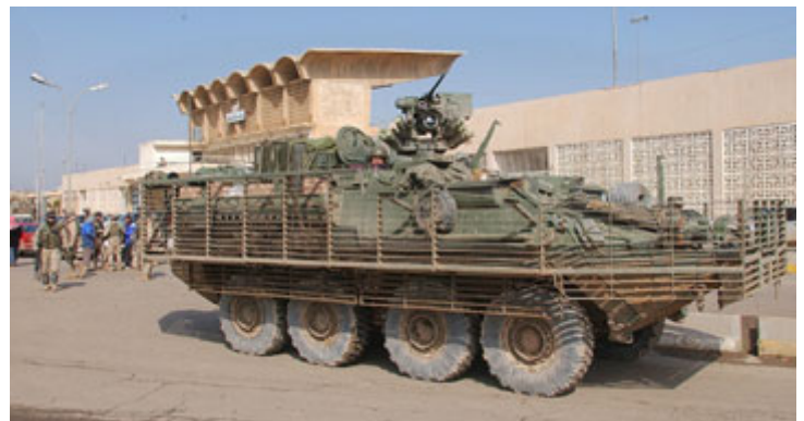
Figure 3: Stryker with protective grating
