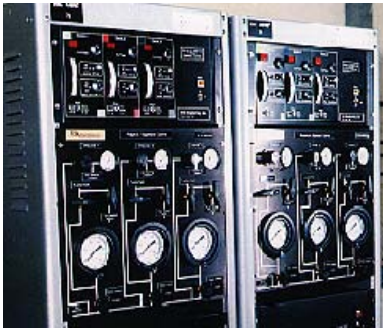
Figure 5 Pneumatic and electronic control rack for 6-device suspension system
