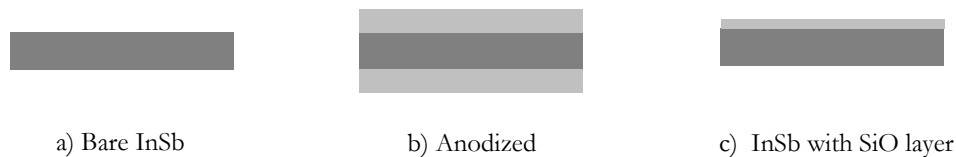
Figure 3.1. Cross view of wafers and their layers.
