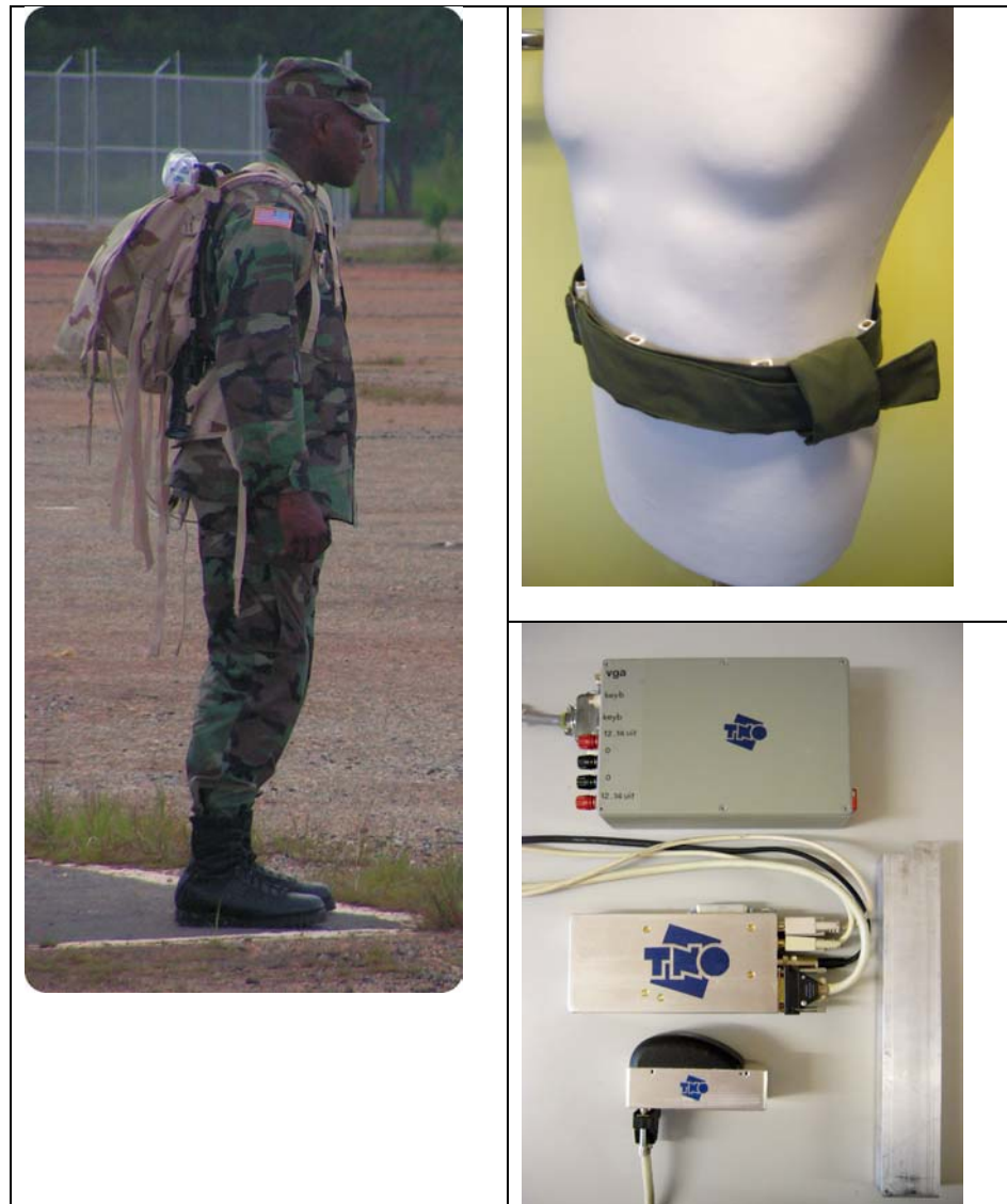
Figure 2.3 – Left: picture of soldier wearing PTN. Top right: picture of the tactile display (waist belt) with the tactors. Bottom right: picture of the PTN system equipment (breakout box, microprocessor, sensor unit, battery unit).
